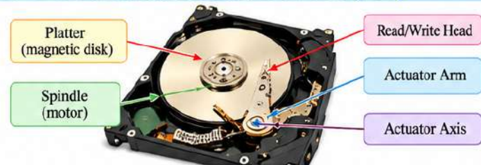
Fig. 3.9 Internal Structure of Hard Disk Drive (HDD)
